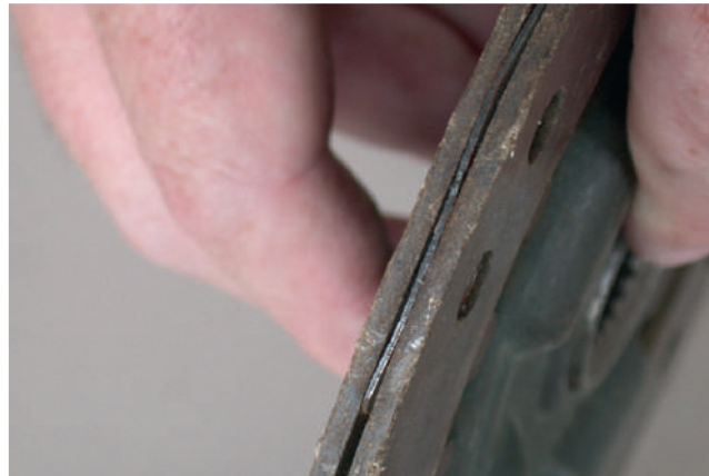
Figure 5.11 Wave springs eliminate chatter
